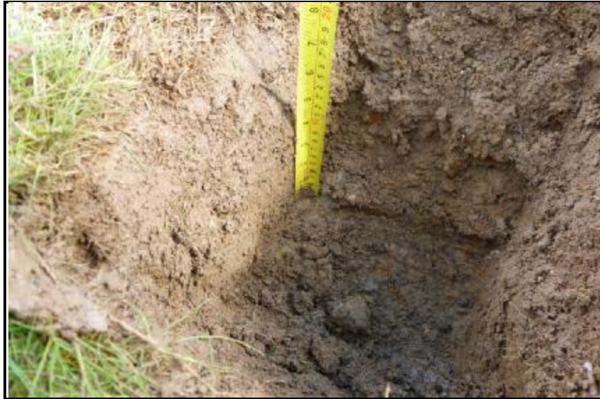
Photograph 5: Trial hole excavation showing depth of clay loam topsoil overlying impervious clay subsoil.
